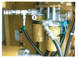
The drain filter (2) is one extra level of contamination prevention Cat excavators offer. Located in the pump compartment behind the pilot filter, the drain filter purifies the case drain from the main pumps, swing motor, and travel motors — all to enhance the life of the pumps and motors and increase uptime for you.
