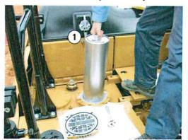
The capsule filter (1) is designed to take out impurities and help you avoid system contamination and accidental spilling. The self-contained, maintenance-friendly filter is easy to remove with a simple wrench. It can take out impurities as small as beta 10 – particles so tiny you cannot see them with the eye. A sensor lets you know if there is a clog or if pressure exceeds a certain level so you can take action.
